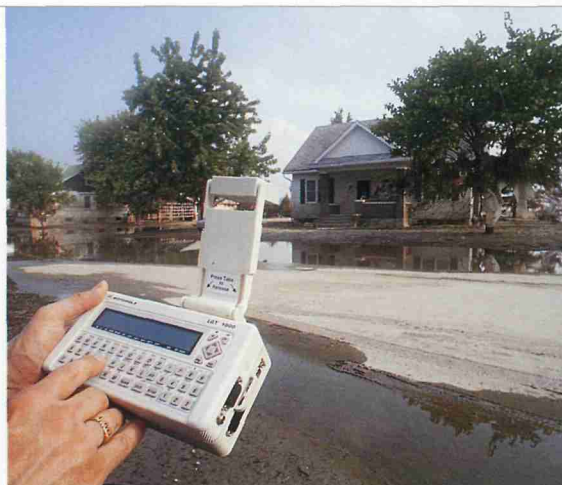
Motorola Global Positioning System equipment was used in surveys to map the extent of the flood damage in Illinois counties along the Mississippi.
