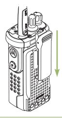
2 To remove the clip, use a flatbladed object to press the belt clip tab (A) away from the radio. Then, slide the clip upward and away from the radio.
