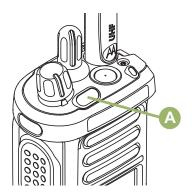
The Top Lightbar indicates the secondary function of MFK and also the status of Intelligent Lighting.
