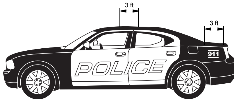
Figure 2-49. Multiple Antennas Separation
