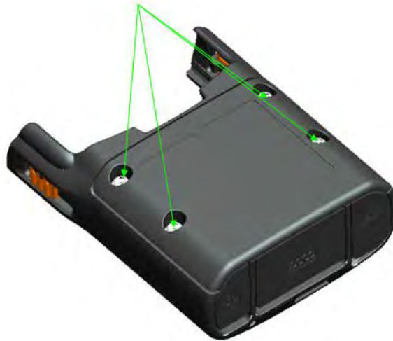
Figure 7-15 Tightening Back Housing
