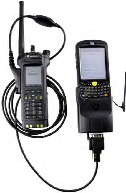
Figure 1-8 KVL and a Portable Radio – Connected (Example)
