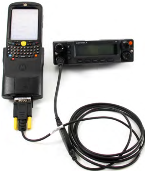
Figure 1-9 KVL and a Mobile Radio – Connected (Example)
